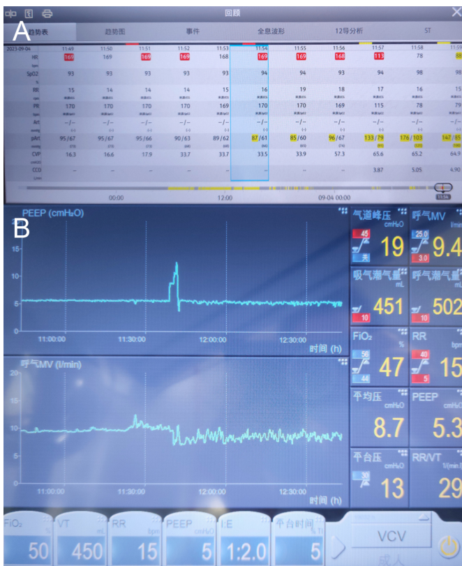
Figure 1: Reversion of SVT to sinus rhythm via high positive end-expiratory pressure (PEEP) during mechanical ventilation. (A) Monitoring of an SVT episode starting at 11:40 (not displayed) and reverting to sinus rhythm by 11:58. It shows changes in heart rate (HR), SpO 2 , and arterial pressure. (B) Gradual increase of PEEP to manage SVT with meticulous monitoring to maintain plateau pressures of less than 30 cm H 2 O.
